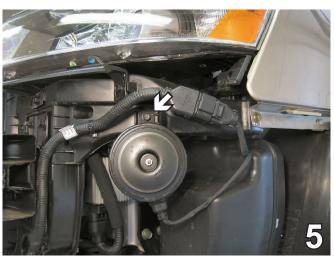
Using a 10MM socket, remove one bolt from the horn bracket, as indicated by the white arrow. Disconnect the wire, as indicated by the grey arrow. Set horn aside to be reinstalled later.
