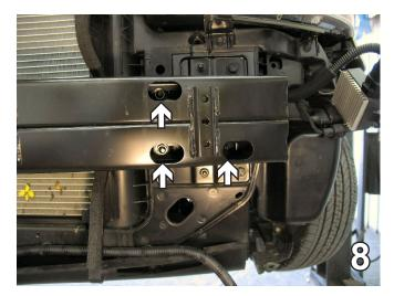
8. Using the 12MM socket, remove three bolts from the metal bumper and set aside to be reinstalled later. Do this to both sides of the vehicle. Release clips and remove air dam from the side of the radiator. Do this to both sides of the vehicle.
