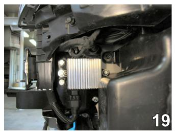
19. Reinstall the fan controller to its original position using the 6MM-1.00 x 45MM hex bolt, 6MM lock washer and four 1/4" flat washers.
