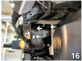
16. On driver's side, insert the 3/8-16 x 1 1/2" hex bolts and 3/8" lock washers into front and upper and lower holes and upper back hole, as indicated by the white arrows in the photo. Insert 3/8-16 x 1" hex bolt and 3/8" lock washer, 3/8" flat washer and 3/8" hex nut into the lower back hole, as shown by the grey arrow in the photo above. Tighten the lower bolt according to the torque specs on the front of these instructions or on page 3 of the Baseplate Towing General Instructions.
