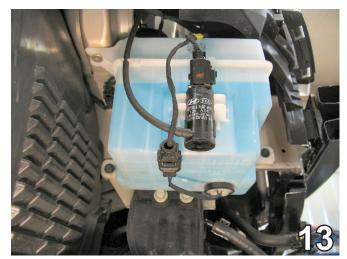
Remove two metric bolts from windshield washer reservoir using the 10MM socket. Unplug electrical connections, disconnect and plug water lines. Set washer reservoir and bolts aside to be reinstalled later.
