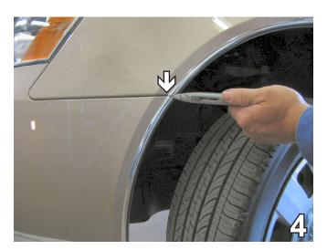
If necessary, use a utility knife to cut the wheel well trim so the fascia may be removed. Pull the front fascia forward and set it aside carefully.
