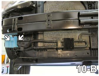
10. Using a reciprocating saw, trim horizontally 2 1/2" just behind the bumper bracket from the outside edge of the radiator support into the frame rail edge. Trim vertically 4" from the bottom, of the radiator support to the horizontal to open area for baseplate installation. Do this to both sides of the vehicle.
