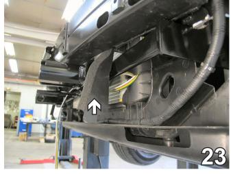
23. Reinstall air dam and trim as needed to fit around the baseplate.
