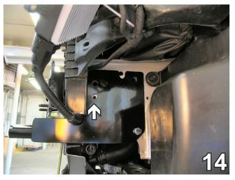
14. Using large vice grips, clamp the baseplate in place by aligning the front, center hole with the existing front hole for the fan controller on the driver's side (see white arrow in photo above). Insure the baseplate is level before clamping on the passenger's side.
