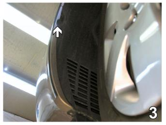
Using a 10MM socket, remove one bolt from the front fascia, inside the wheel well. Do this to both sides of the vehicle. Set bolts aside to be reinstalled later.
