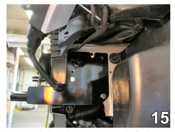
15. Using the baseplate as a template, drill five holes in the baseplate endplate with the 13/32" drill bit. Do this to both sides of the vehicle, the driver's side is shown.
