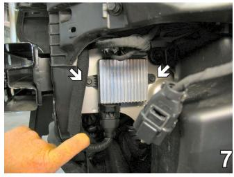
On the driver's side, just behind the metal bumper, remove two bolts with the 10MM socket and set the fan controller and bolts aside to be reinstalled later.
