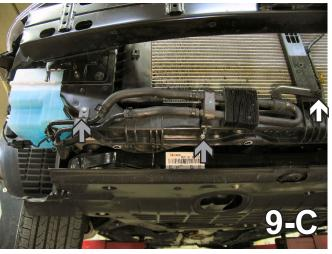
Using the 10MM socket, remove three bolts from coolant tubing (see 9-A). Relocate driver's side bolt to lower existing threaded hole in coolant tubing bracket. Bend middle coolant tube bracket 90 degrees toward the radiator (see 9-B). Refasten using two self drilling screws (gray arrows). Photo 9-C shows relocated coolant tubing.
