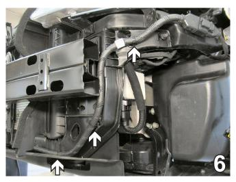
6. Remove three clips from electrical cable. Move the cable aside to clear area for baseplate installation.
