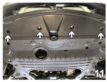
11. Using a 10MM socket, remove four bolts underneath the belly pan. Pull the belly pan forward and set aside to be reinstalled later.
