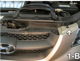
Remove seven Phillips screws from the top edge of the front fascia, as indicated by the white arrows in photo 1-A. Remove two bolts from the top side of the fascia using a 10MM socket, as indicated by the arrow in photo 1-B. Set push pins and bolts aside to be reinstalled later.
